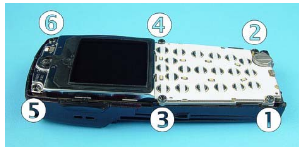
7) Unscrew the six Torx PLUSÆ size 6 screws. For assembly, the reverse order and a torque driver with a torque of 20Ncm have to be used.
