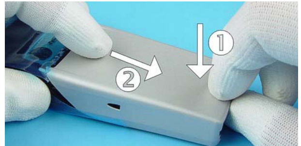
3) Press the Release Button before pulling up the B-Cover .
