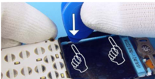
15) Remove the LCD Module by using SRT-6 as shown in the picture.
