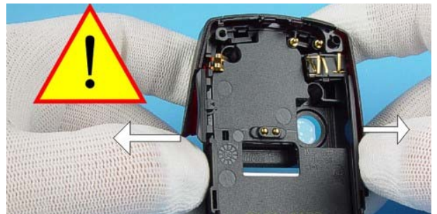
19) Spread the B-Cover from both sides until snaps inside will release it.
