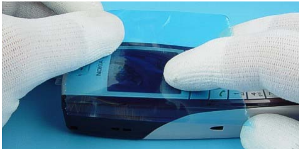
2) Check the condition of the window and protect the window with a film.
