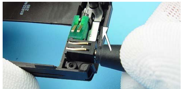
21) A DC plug can be used to remove the DC Jack.
